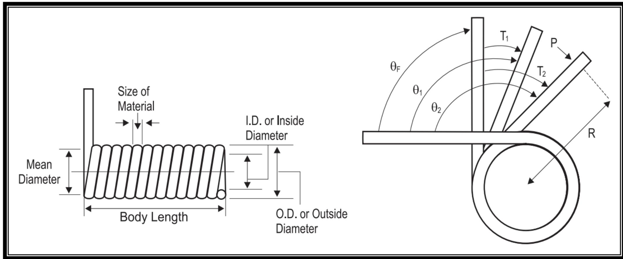
**Figure ST-14. Helical Torsion Spring Definitions.**
