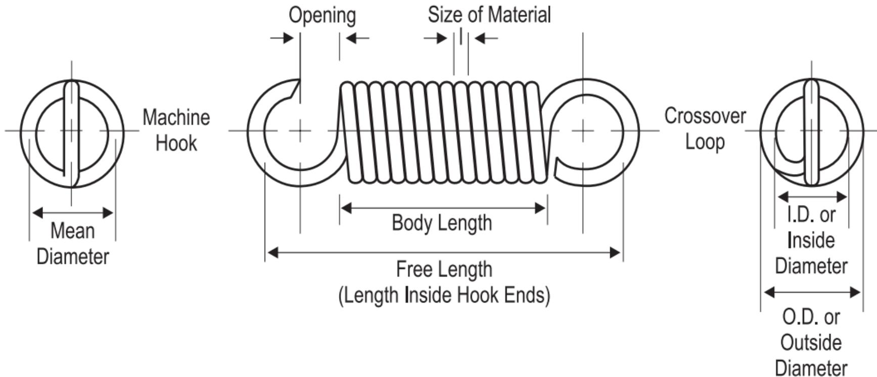
**Figure ST-10. Helical Extension Spring Definitions.**
